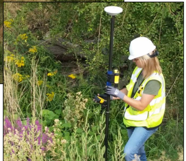
Engineering Technician gathers GPS coordinates on water, sewer and storm valves and manholes which were missing from off the City's utility maps.
