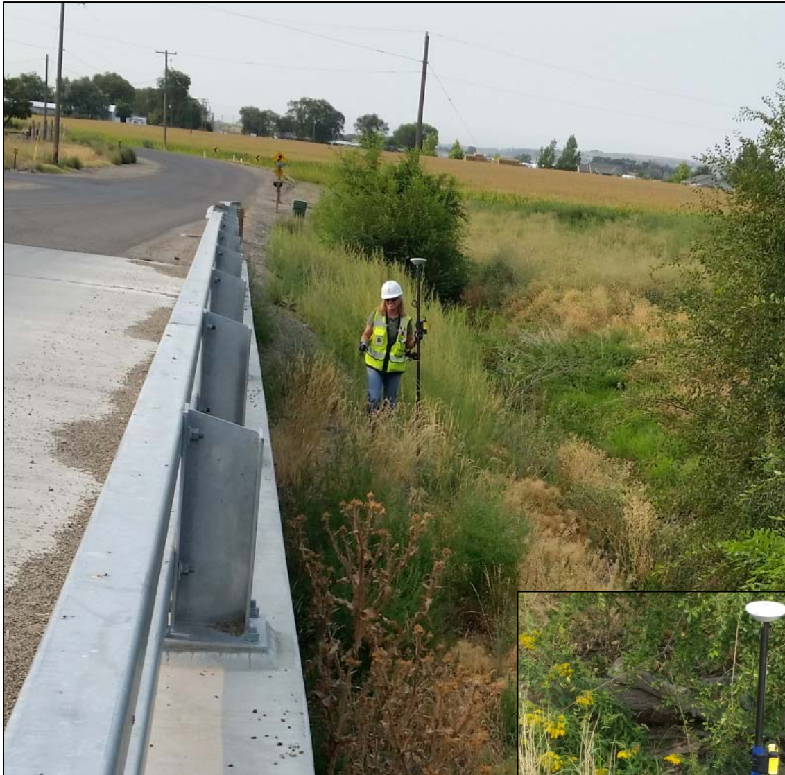
Engineering Technician gathers GPS coordinates on water, sewer and storm valves and manholes which were missing from off the City's utility maps.
