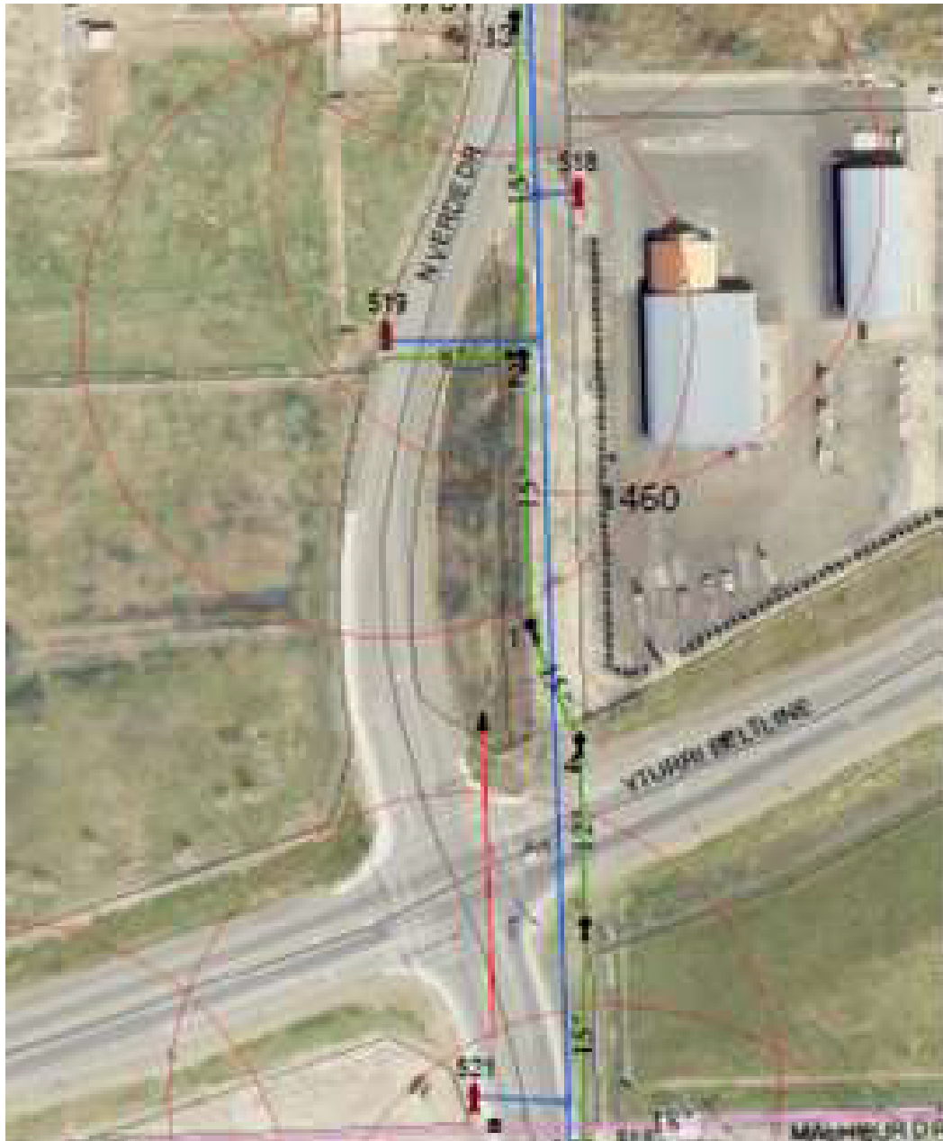
Figure 4 Sewer and Water Lines Serving Subject Properties
