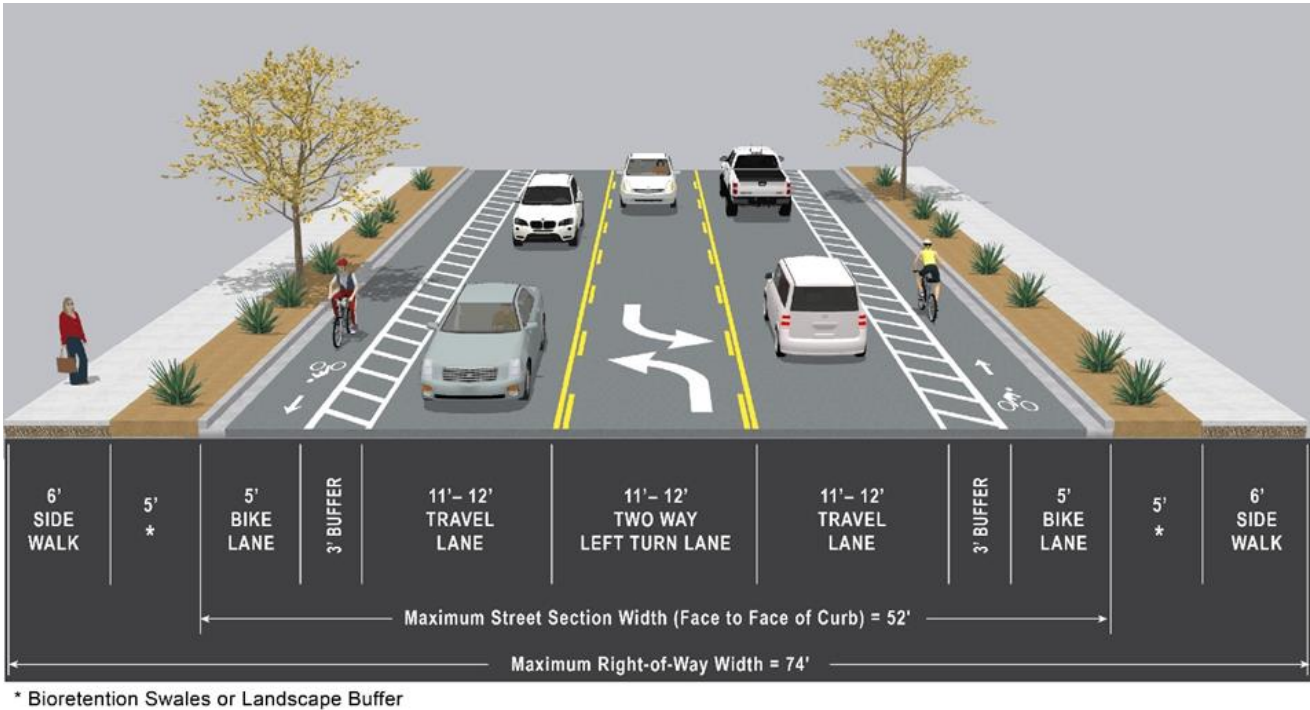
Figure 5 Three-Lane Minor Arterial Cross-Section
