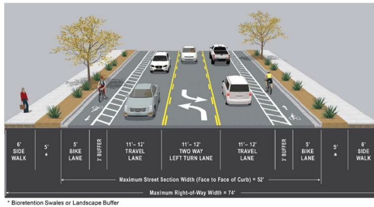
Figure 10C-25.08c – Three-Lane Minor Arterial
