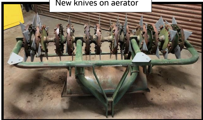
New knives on aerator
