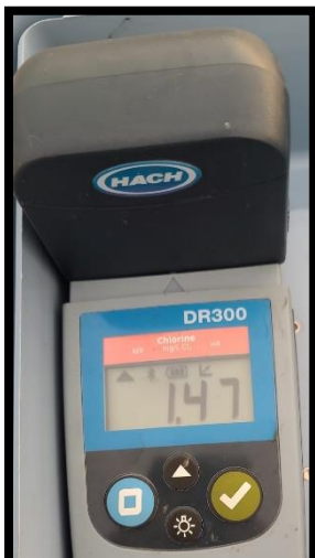
Chlorine residual after water main repair at SW 3 rd Ave and SW 4 th St.
