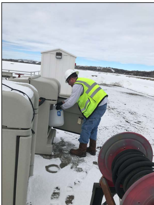
Operator installing a vessel to collect a 24 hour composite sample at the Wastewater Treatment Plant for effluent Biological Oxygen Demand (BOD) and Total Suspended Solids (TSS) monitoring.
