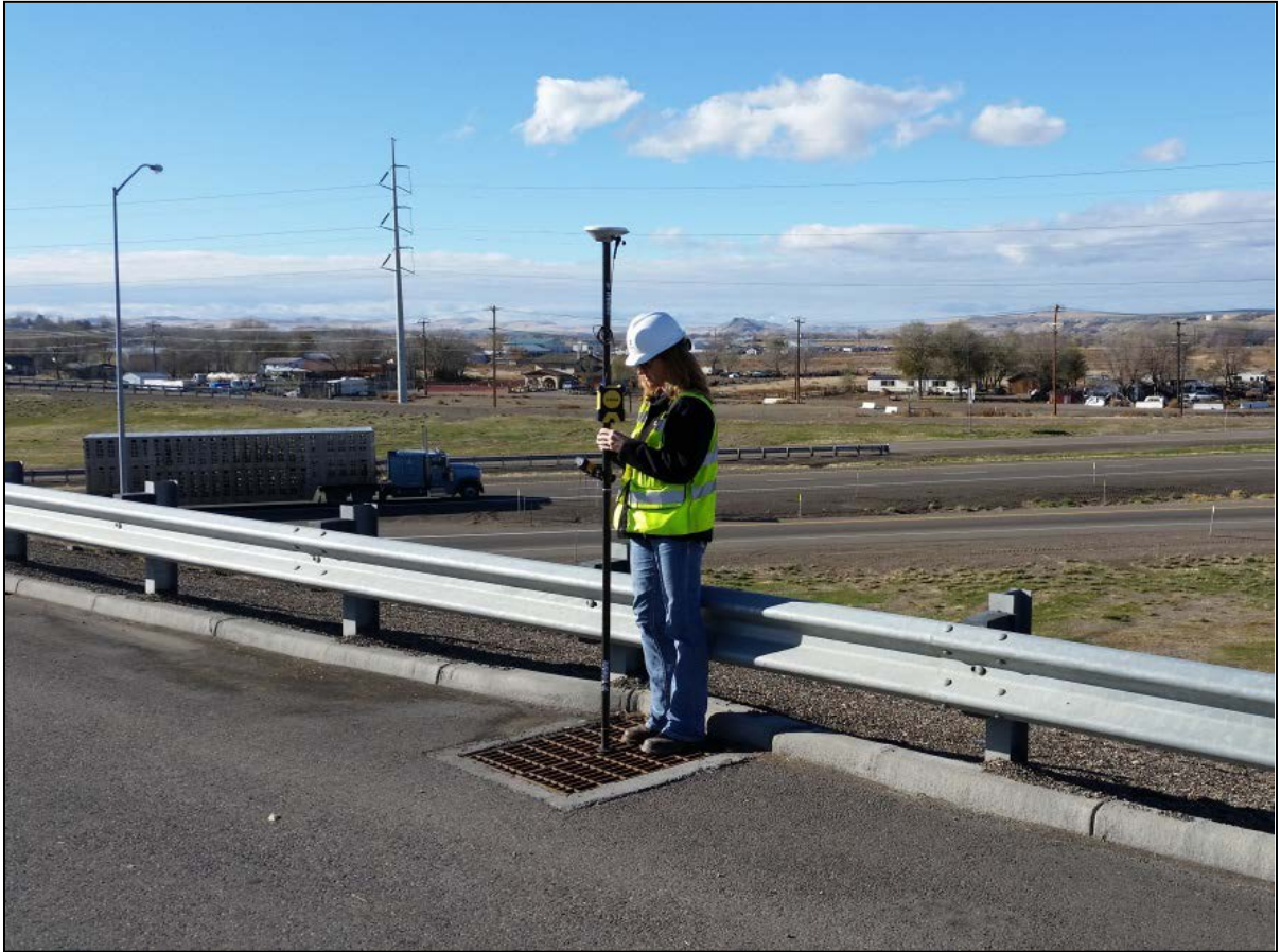
Engineering Technician utilizes a Global Positioning System (GPS) handheld unit to collect a point on a catch basin on the Highway 201 Interstate 84 overpass.
