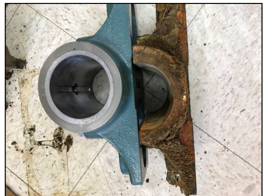
Bearing repair at Water Treatment Plant – new and replaced bearing pictured above.
